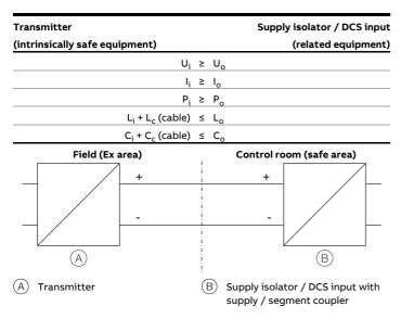
Figure 1: Intrinsic safety installation check
