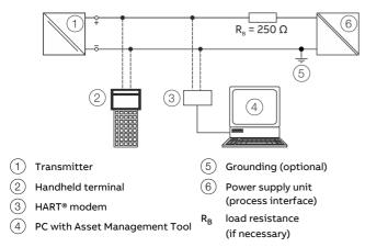
Figure 13: Example for HART connection
