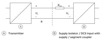
Figure 12: HART load resistance
